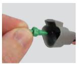
**Step 4:**Once all contacts are in place, insert green wedge. The green wedge will snap into place.
