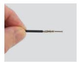
**Step 1:** Grasp crimped contact approximately one inch behind the contact barrel.
